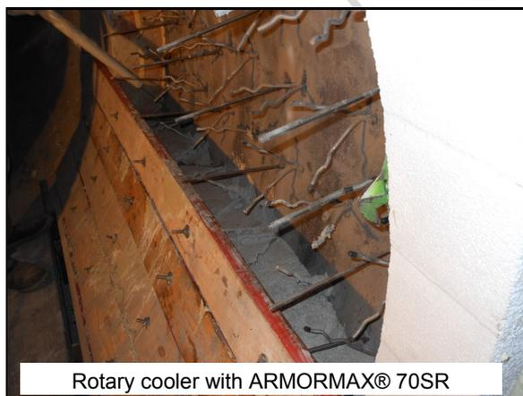
Rotary cooler with ARMORMAX® 70SR
