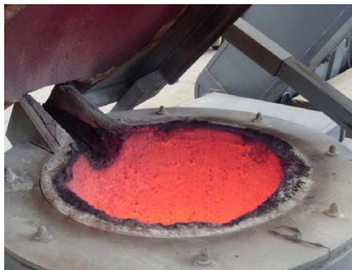
Figure 1 – Iron melting coreless furnace with silica lining
