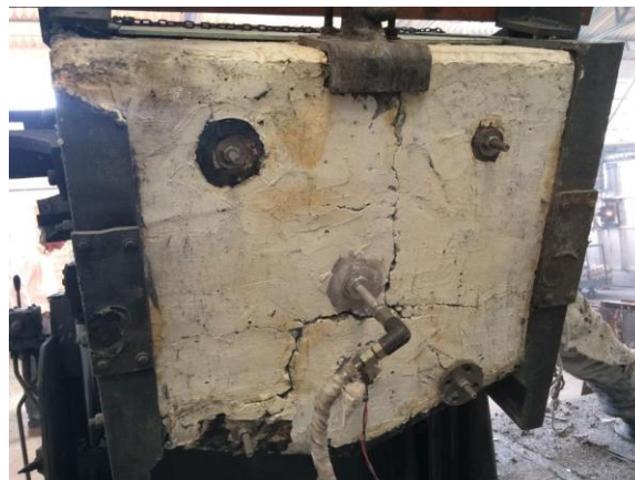
Figure 2 - Bottom block cracked
