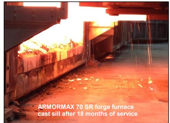
ARMORMAX 70 SR forge furnace cast sill after 18 months of service
