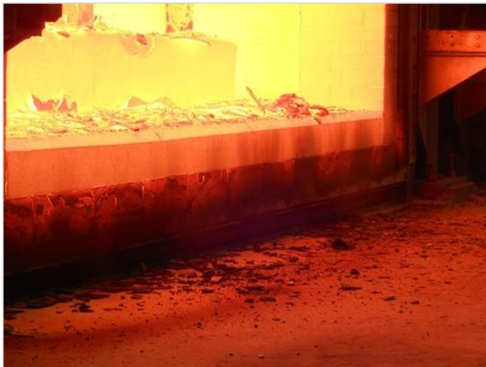
ARMORMAX® sill after 1 month in service
