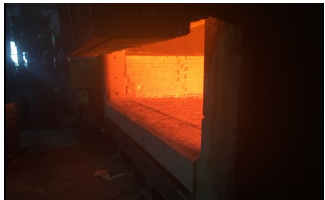
ARMORMAX® sill after 52 months in service
