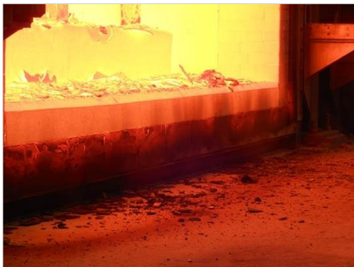
ARMORMAX® sill after 1 month in service
