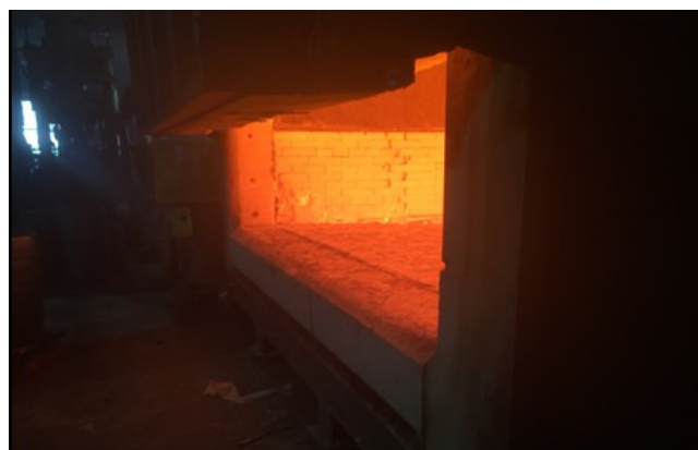
ARMORMAX® sill after 52 months in service
