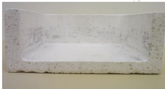
WAM® AL III vessel after metal has been removed
