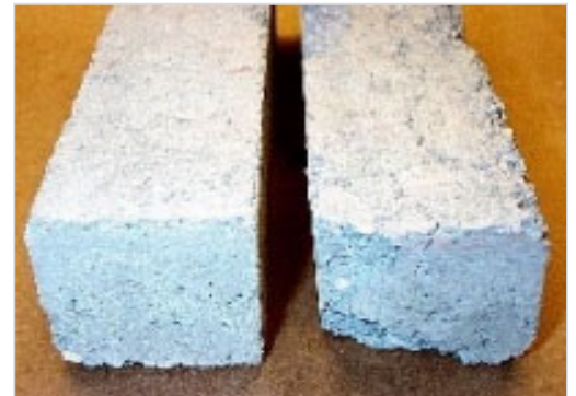
TUFFLOOR® Standard Concrete Thermal Cycling to 760°C (1400°F)
